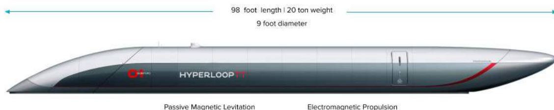
Exhibit 2-3: Capsule Prototype, Courtesy of HyperloopTT
