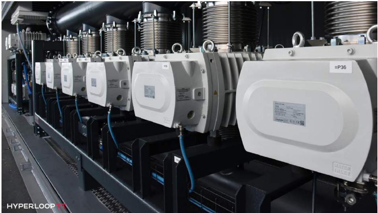
Exhibit 2-8: Vacuum pumps and modular housing, Courtesy of HyperloopTT
